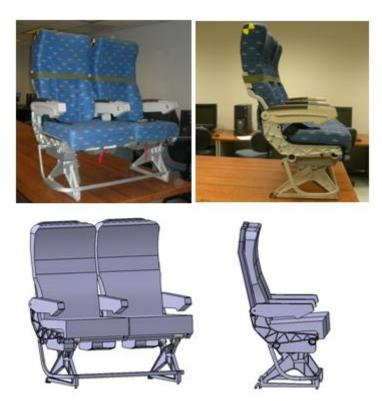
Figure 5 Comparison of Actual Seat and CAD Model
