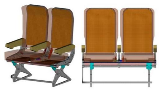
Figure 6 FE Model of Typical Aircraft Seat
