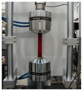
Figure 2 Seat Belt Test Setup (NIAR Test Facility)
