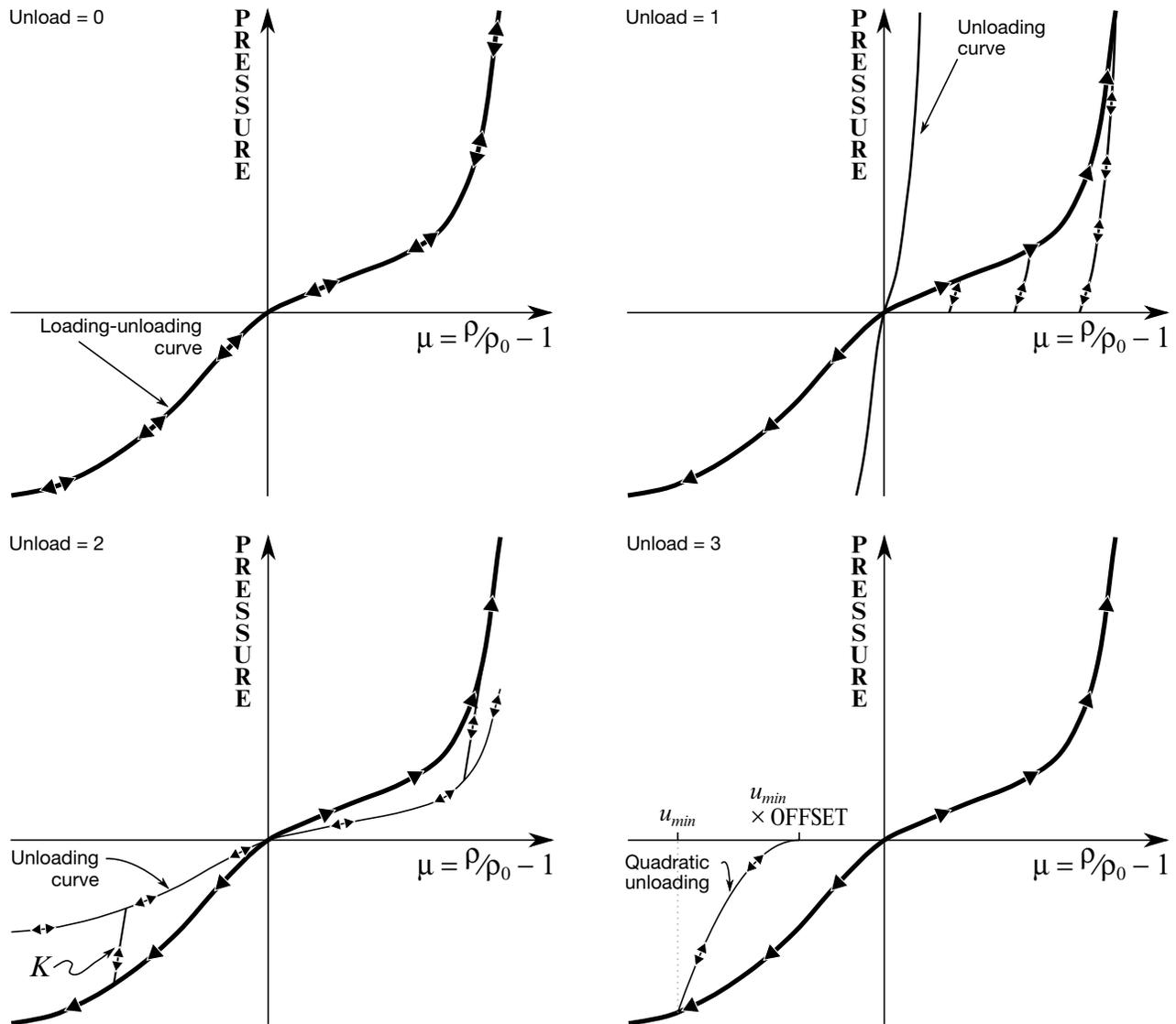
Figure EOS15-1. Load and unloading behavior.
