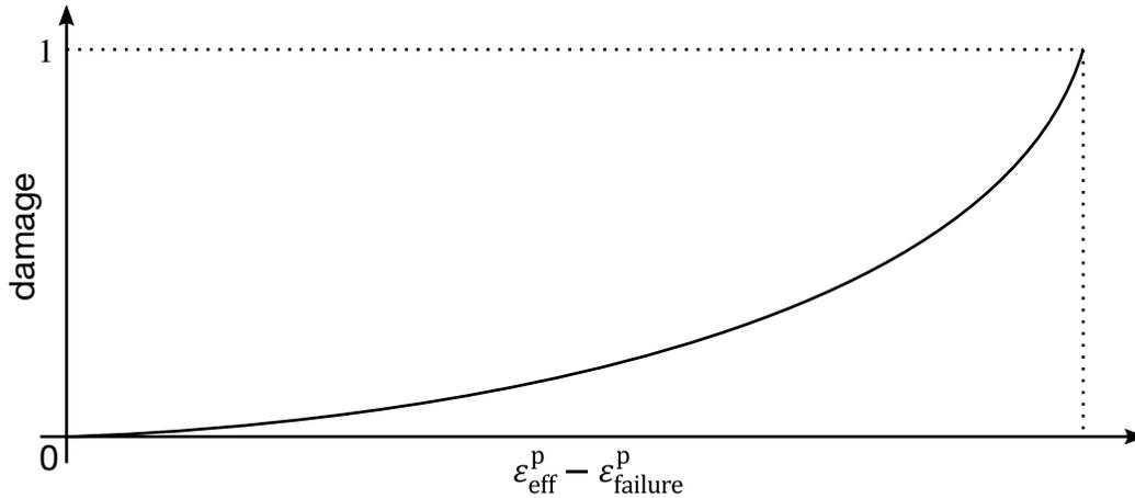
**Figure M81-2.** A nonlinear damage curve is optional. Note that the origin of the curve is at (0,0). The nonlinear damage curve is useful for controlling the softening behavior after the failure strain EPPF is reached.
