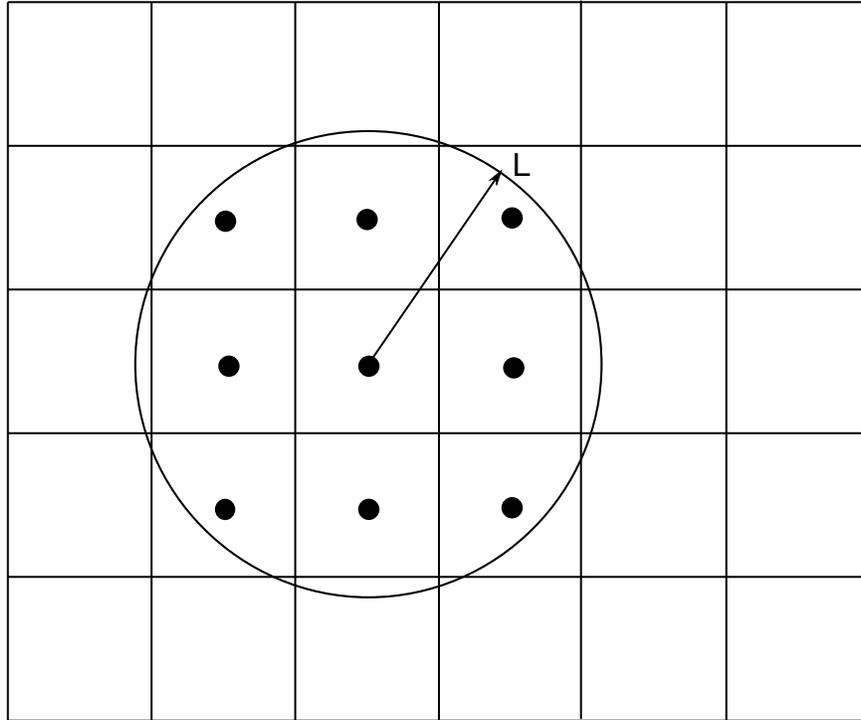
**Figure 2-4.** Here  $\dot{f}_r$  and  $x_r$  are respectively the nonlocal rate of increase of damage and the center of the element  $e_r$ , and  $\dot{f}_{local}^i$ ,  $V_i$  and  $y_i$  are respectively the local rate of increase of damage, the volume and the center of element  $e_i$ .
