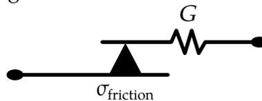
Several springs and sliders in series can be defined that are put in parallel to the rest of the stress contributions of this material model.
