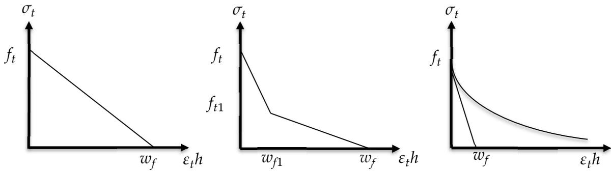
The variable  $h$  is a mesh-dependent measure used to convert strains to displacements. The variable  $\epsilon_t$  is called the inelastic tensile strain and is defined as the sum of the irreversible plastic strain  $\epsilon_p$  and the reversible strain  $w_t(\epsilon - \epsilon_p)$  (in compression  $w_c(\epsilon - \epsilon_p)$ ). To get the influence of multi-axial stress states on the softening a damage ductility measure  $x_s$  is added:
