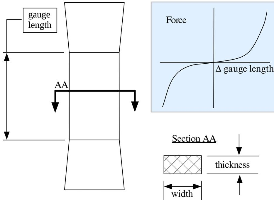
Figure M27-1. Uniaxial specimen for experimental data
