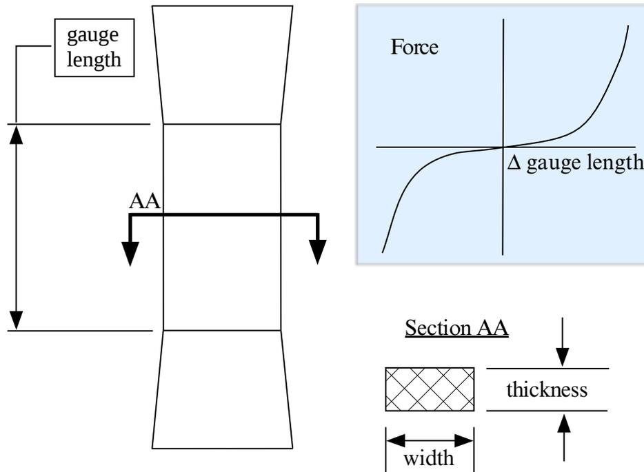
Figure M218-1. Uniaxial specimen for experimental data
