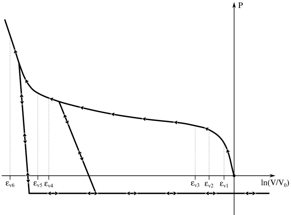
**Figure EOS8-1.** Pressure as a function of volumetric strain curve for Equation of State Form 8 with compaction. In the compacted states the bulk unloading modulus depends on the peak volumetric strain. Volumetric strain values should be input with correct sign (negative in compression) and in descending order. Pressure is positive in compression.
