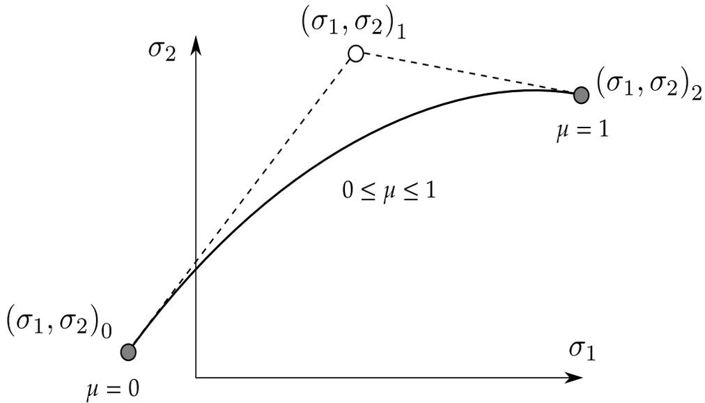
Figure M136-1. Bézier interpolation curve.
