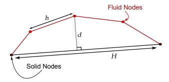
**Figure 5-1.** Geometry of FSI contact.
