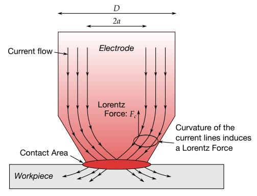
**Figure 4-3.** Electrode coming into contact with workpiece (RSW application).
