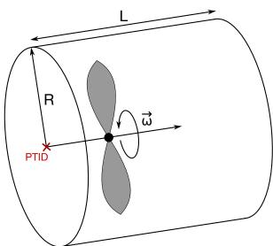
**Figure 5-2.** Non Inertial Reference Frame Example
