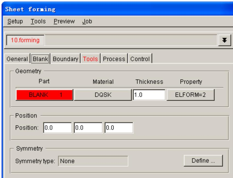
Figure 2.18 Blank definition interface
