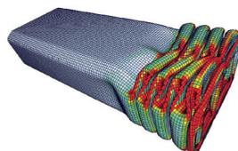
Simulation of Short Fiber Reinforced Composites
